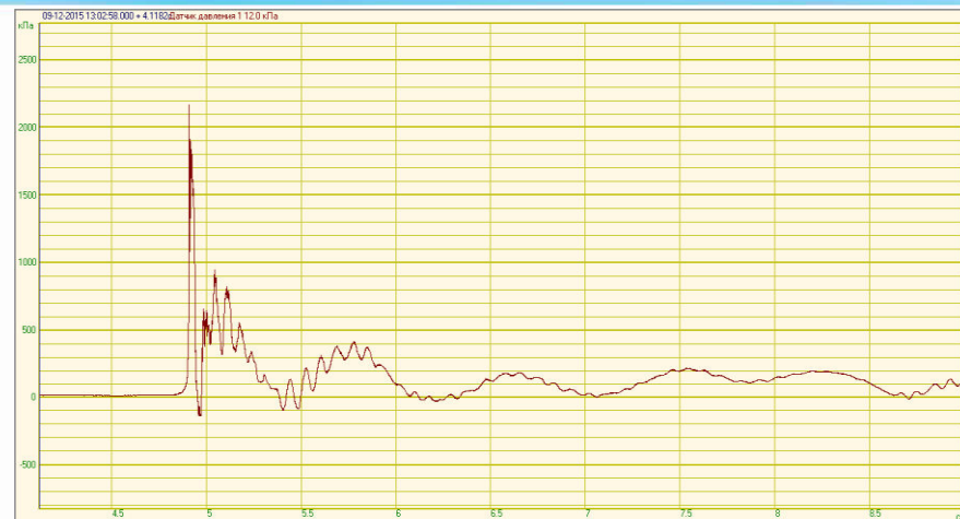
Picture 1 – Water hammer without PA (Dn 200)
