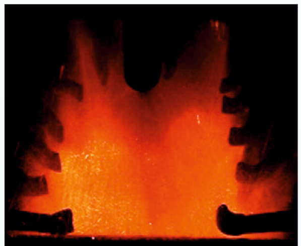
Coal-water fuel burning in the fluidized bed
